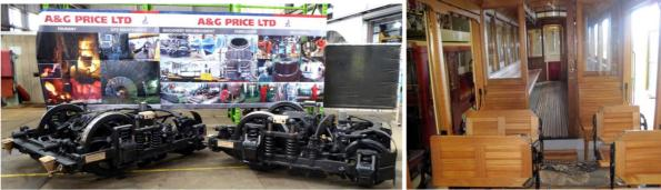
Mechanical work, such as fitting the trucks to the tram body, the hand brake standards and mechanisms, trolley pole pedestal and fittings, sand box mechanisms and other fittings were fitted at the Museum. The hand-brake pedestals and gearing mechanism were manufactured by local firm Tunley Engineering Ltd. of Paraparaumu. The Ackley brake mechanisms are ex Ballarat. All final assembly and finishing work was completed by Museum members
