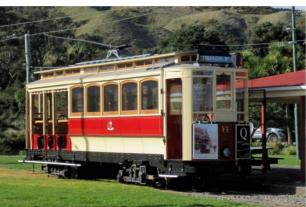
No. 17, which had started life as a small, single-truck, single saloon tram had been converted in 1911 to a double-truck combination tram. The 5-window length single saloon was placed on one end of a new, longer chassis and the remaining one third of the chassis became the open portion of a "new" double truck combination tram. The tram body remained on a Raumati South property, used as
